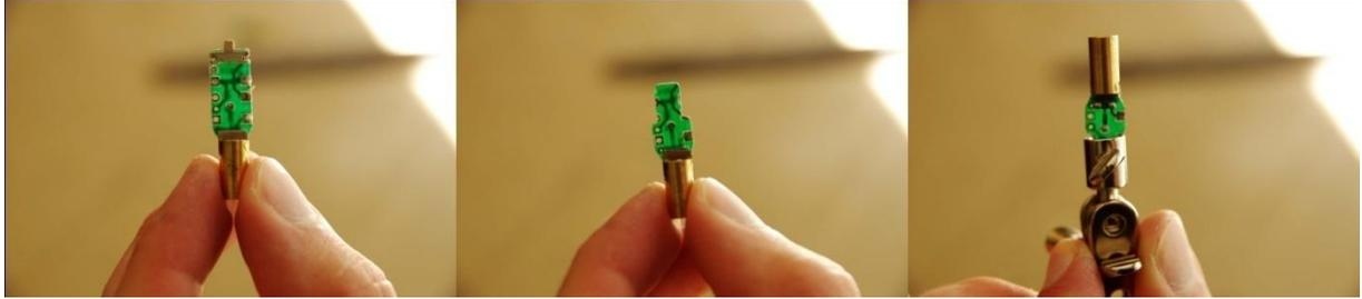
Solder in series three 1,5V batteries.
