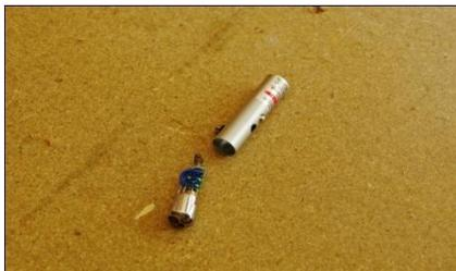
Take of the cap, and unsolder the unwanted elements. (on ours we had two LEDs and two push button)
