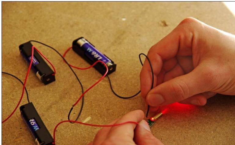
Solder two cables of about 10cm long on each pole.
