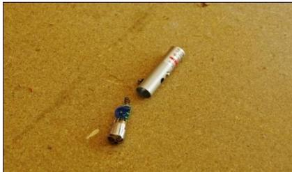
Take of the cap, and unsolder the unwanted elements. (on ours we had two LEDs and two push button)
