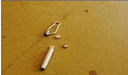
Pull out the top cap which should hold the laser and a small printed circuit board.
